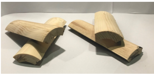
A FORSTNER WAS USED TO DRILL A LARGE HOLE IN THE MIDDLE OF THE CYLINDER—THIS WAS DRILLED IN FROM BOTH SIDES (ONE AT A TIME) DUE TO THE LENGTH OF THE BIT BEING SHORTER THAN THE LENGTH OF THE WOOD.
