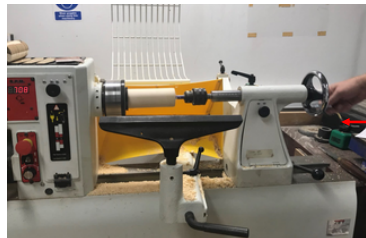
A FORSTNER WAS USED TO DRILL A LARGE HOLE IN THE MIDDLE OF THE CYLINDER—THIS WAS DRILLED IN FROM BOTH SIDES (ONE AT A TIME) DUE TO THE LENGTH OF THE BIT BEING SHORTER THAN THE LENGTH OF THE WOOD.
