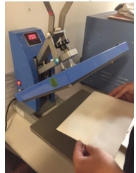
PRINTED PAPER IS PLACED ON TO THE HEAT PRESS AND THE TIME IS SET.
