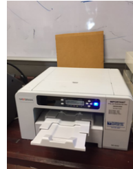
LOGO IS PRINTED OUT USING A SPECIAL PRINTER FOR SUBLIMATION, ON SPECIAL PAPER.
