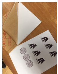
WHEN THE LOGO IS PRINTED, IT MUST BE INVERTED BECAUSE THE PICTURE PRINTED WOULD BE LIKE LOOKING INTO A MIRROR.
