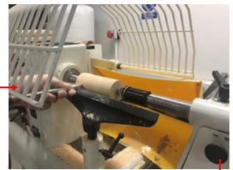
THEY WERE PUT ON THE WOOD TURNING LATHE MACHINE AND ARE TURNED INTO A CYLINDRICAL FORM.
