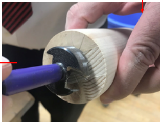
A FORSTNER WAS USED TO DRILL A LARGE HOLE IN THE MIDDLE OF THE CYLINDER—THIS WAS DRILLED IN FROM BOTH SIDES (ONE AT A TIME) DUE TO THE LENGTH OF THE BIT BEING SHORTER THAN THE LENGTH OF THE WOOD.
